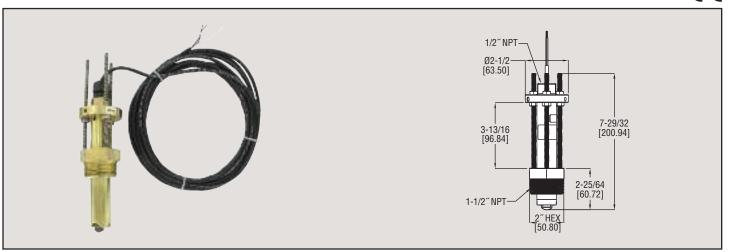
The Series PFT is a paddlewheel flow sensor used to monitor liquid flow rates in pipes from 1-1/2 to 40 " with just one size adjustable sensor. Multiple wetted material choices offer application versatility. The PFT is ideal for monitoring water flow rates in irrigation systems and building automation cooling systems.
